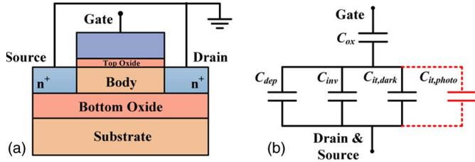
Fig. 2. (a) SOI MOSFET structure and (b) its equivalent capacitive circuit model with a subbandgap optical illumination for SODBoF technique.  $C_{it,photo}$  is the capacitive component originated from the photoexcited carriers from the photoresponsive traps.
