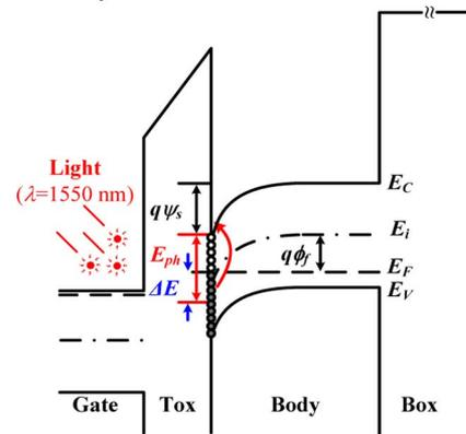
Fig. 1. Energy band diagrams under subbandgap ( $E_{ph} < E_{g,Si}$ ) optical illumination in n-channel SOI MOSFETs. The trapped electrons within the photoresponsive energy ( $E_C - E_{ph}$ )  $< E_t < (E_i - q\varphi_f \pm q\psi_s)$  are excited to the conduction band and contribute to the drain current.
